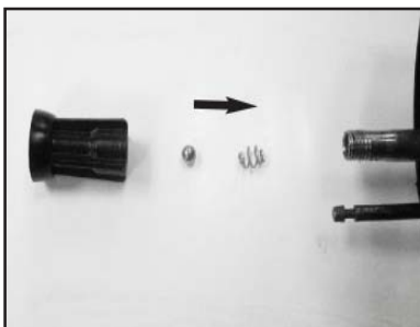
8. Install ball (161008) and spring (161010) into piston (181131). Thread piston assembly back into place.
