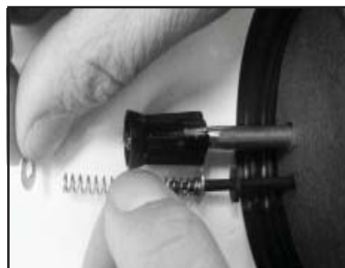
9. Install new rod gasket (161013), first rod washer (161065), rod spring (161014), then second rod washer (161065).
