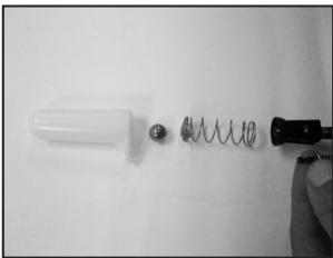
10. Install cylinder ball (161009) and cylinder spring (161011) into cylinder (161006).
