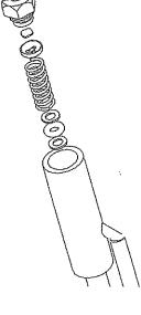
To replace pump parts, unscrew check valve on end of pump and remove spring; O-ring and two washers.
