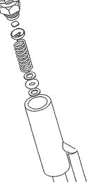
To replace pump parts, unscrew check valve on end of pump and remove spring; O-ring and two washers.
